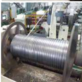
▲ 套筒料加工 Continuous rolling of bush material
