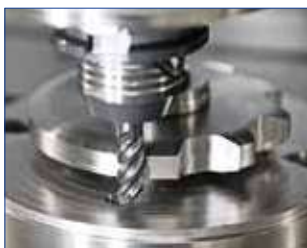
Sprocket manufacturing on CNC machines
